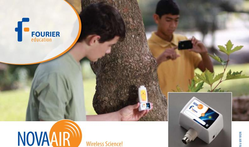
NOVA AIR ™ a compact wireless one channel data logger designed to transmit data from Fourier's sensors to computers and iOS devices (iPad / iPhone / iPod Touch). With NOVA AIR, teachers and students have the ability to conduct a wider range of scientific experiments that were previously unapproachable due to the limitations of cables and cords.
