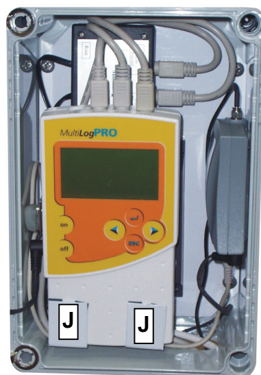
Figure 18: MultiLogPRO inside the Weather Station main box
