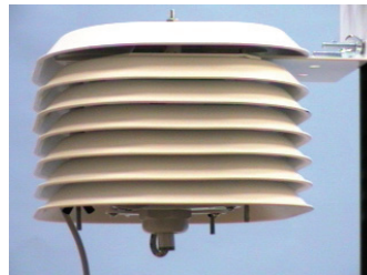
Figure 4: Radiation shield with the temperature and humidity dual sensor mounted inside
